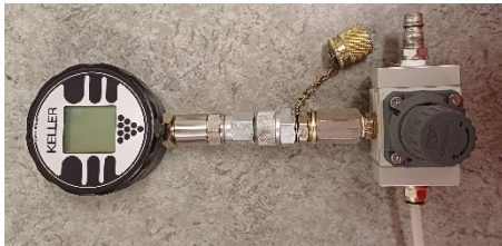
Picture 5. Digital pressure gauge with manual adjustment valve, d=0,001\text{MPa} .
