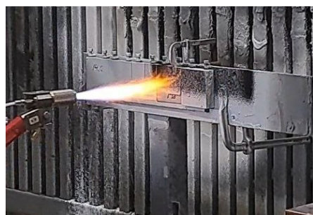
Picture 3 Flame spraying of PE at Tampere University's Thermal Spray Laboratory.
