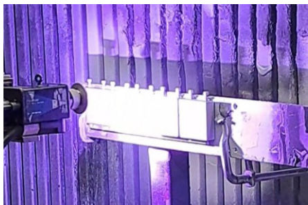
Picture 2 Electric arc spraying of Zn at Tampere University's Thermal Spray Laboratory.
